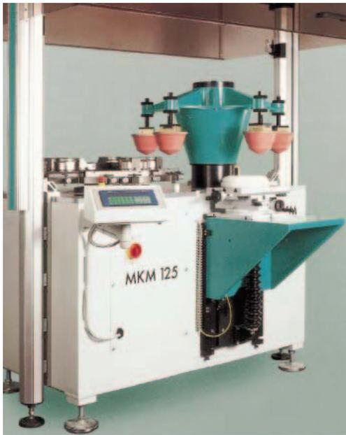
Gambar 6.25. Mesin cetak pad multicolor carousel (MKM 125, Morlock)
