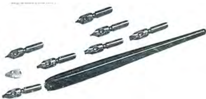
Gambar 6. Pena gambar/pen kodok Sumber: Caldwell, Peter, 1993, Pen & Ink Sketching , London, B.T. Batsford Ltd
