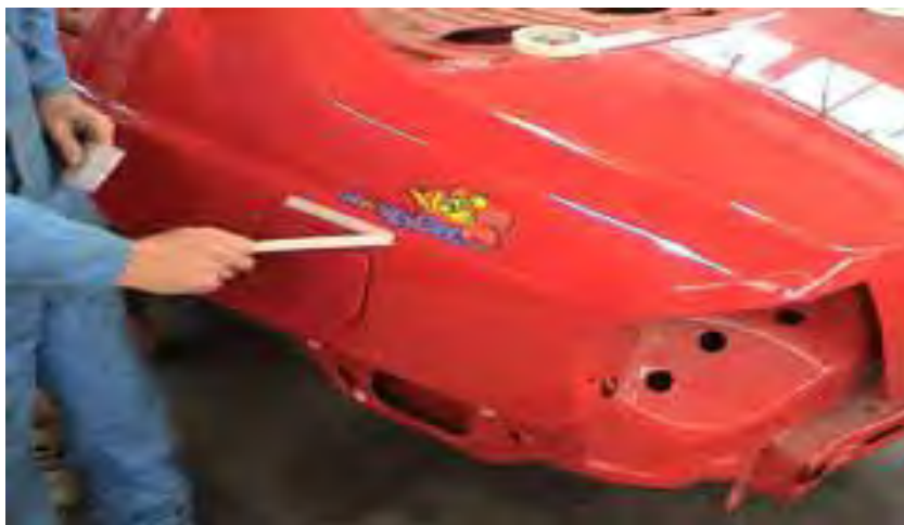
Gb.2.54. Pelepasan masking tape penanda
