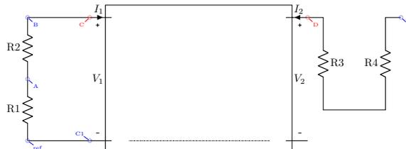
Fitting some circuit inside the Quadripole (nodes C and E):
