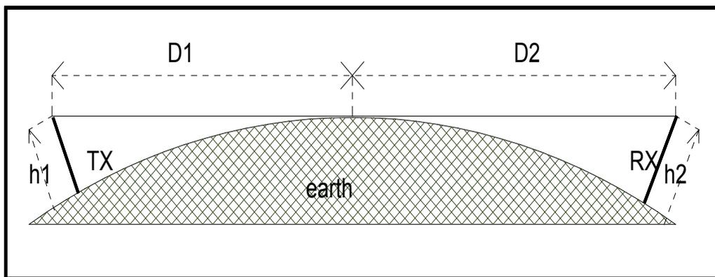
**Fig 3.4.** The maximum line-of-sight distance between two elevated antennas is equal to the sum of their distances to the horizon. Total reachable distance is equal to the sum of D1 and D2.
