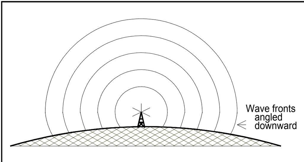
**Fig 3.2** The surface-following property is caused by retarding the velocity of the wave at the surface boundary. The retarding due to the earth's absorption will angle the wave fronts downwards.
