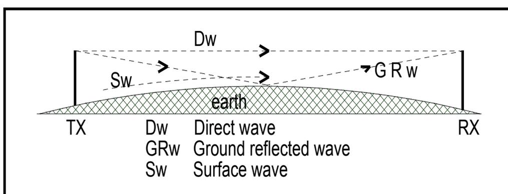
**Fig. 3.1** Ground waves can be direct, be ground reflected, or follow the surface.
