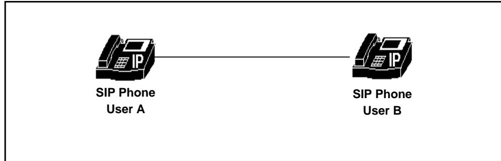
**Figure 1-2. Basic Connection Between Two SIP Phones**
