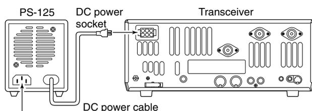
Connect to an AC outlet using the supplied AC cable.
