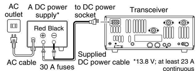
**NOTE:** Although the power supply current requirement is quite low during receiving, this not the case when you transmit. With many electrical devices in the shack, it is very important to verify the electrical circuit is not overloaded.
