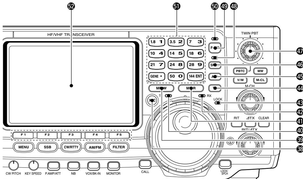
**38 TRANSMIT FREQUENCY CHECK SWITCH [XFC]** (pgs. 45, 48)
