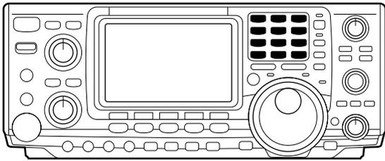
• Say you want to go to 20 meters or 14 MHz; you would push the [14 5]. This will immediately change the displayed operating frequency to the 20-meter band. By pushing [14 5] again, frequency pre-sets in the triple band stacking registers frequency can be displayed. For more details on this system refer to p. 19.
