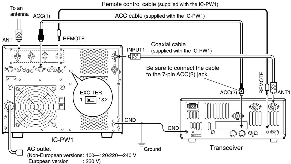
Turn OFF the transceiver's antenna tuner while tuning the IC-PW1's tuner.
