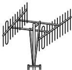
Connect a VHF (60–144 MHz) antenna; impedance: 50 Ω.
