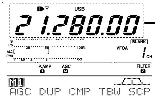
In this example, pushing [MP-W] enters 21.28000 MHz USB into the top memo pad and erases the oldest memo pad (21.34724 MHz LSB).
