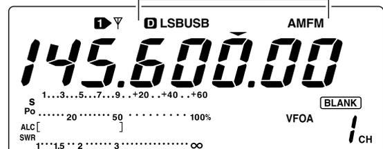
**NOTE:** When connecting a TNC to the ACC socket on the rear panel, select SSB (LSB/USB) data mode or disconnect the microphone and rotate [MIC GAIN] fully counterclockwise.
