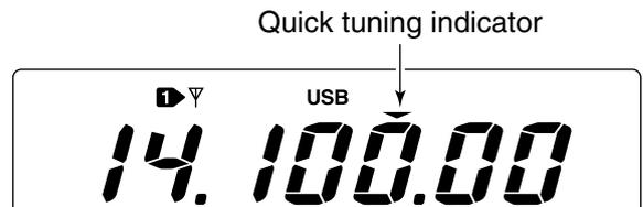
➔ While the quick tuning step is OFF, turns the 1 Hz step ON and OFF when pushed for 1 sec.
