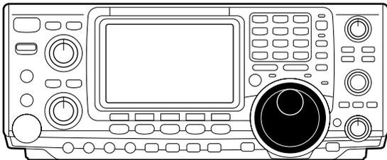
**NOTE:** Although you can directly enter the frequency with the keypad, using the Band Stacking Register and the tuning knob is the most popular method of hopping around the bands. For more information regarding the direct frequency entry method, refer to p. 22.
