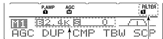
The selected filter width is indicated for approx. 1 sec. when [FILTER] is pushed.
