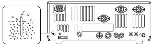
**WARNING!** NEVER ground station equipment or antennas to house gas lines. NEVER attach ground lines to plastic (pvc) pipe.
