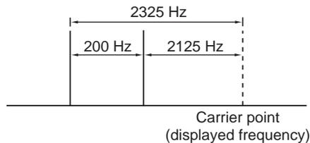
**NOTE:** When SSB data mode is selected, the audio input from the **[ACC(1)]** (pin 6) is used for transmission instead of **[MIC]**'s.
