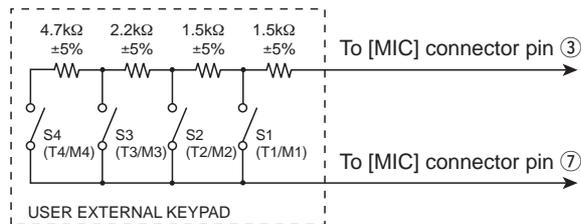
**Auto** Pushing one of external keypad switches, transmits the desired voice memory during a phone mode (SSB, AM or FM), or memory keyer contents during CW mode operation.
