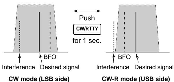
CW-R (CW Reverse) mode receives CW signals with a reverse side CW carrier point like that of LSB and USB modes.
