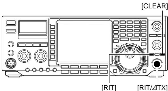
When RIT and  $\Delta$ TX are ON at the same time, the [RIT/ΔTX] control shifts both the transmit and receive frequencies from the displayed frequency at the same time.
