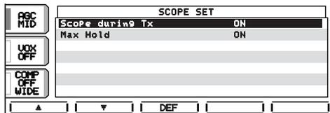
The spectrum scope shows the transmit signal waveform while transmitting. This can be deactivated if desired.
