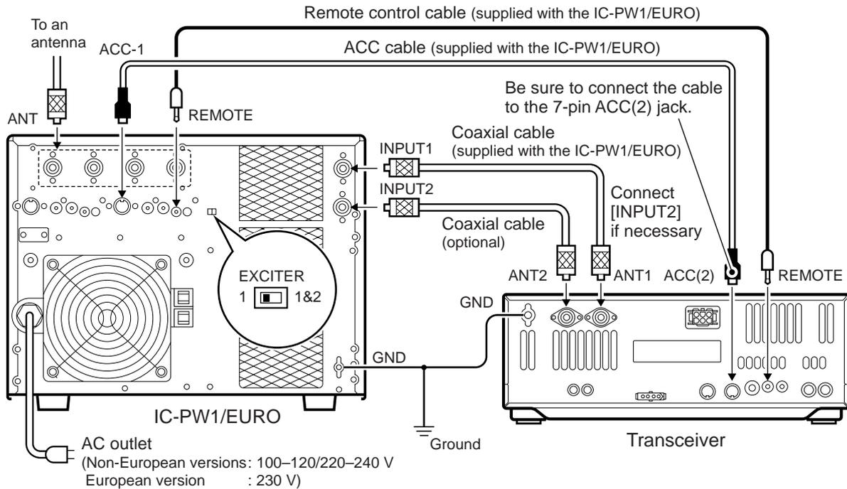
Turn OFF the transceiver's antenna tuner while tuning the IC-PW1/EURO's tuner.
