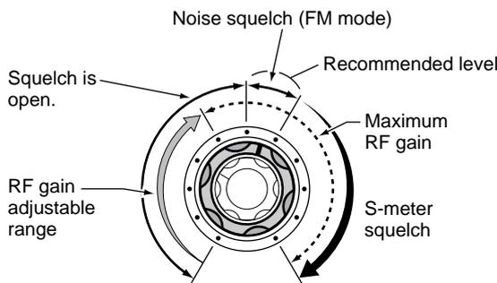
**•When functioning as RF gain control**
