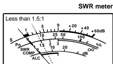
▨ The built-in antenna tuner matches the transmitter to the antenna when the SWR is lower than 3 : 1.
