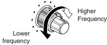
The received CW audio pitch and monitored CW audio can be adjusted to suit your preference (300 to 900 Hz in 25 Hz steps) without changing the operating frequency.
