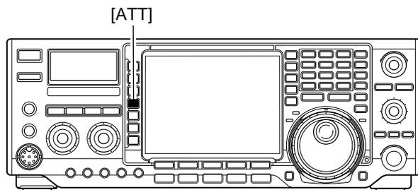
➔ Push **[ATT]** several times to set the attenuator 6 dB, 12 dB, 18 dB or OFF.
