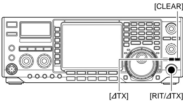
When RIT and ΔTX are ON at the same time, the [RIT/ΔTX] control shifts both the transmit and receive frequencies from the displayed frequency at the same time.
