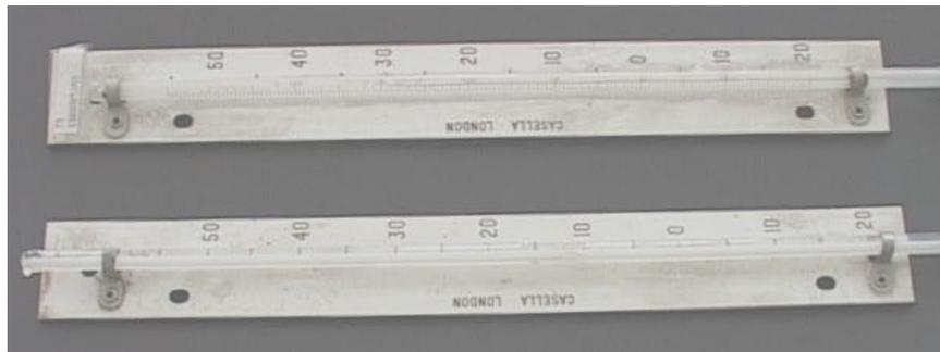
**Sketsa thermometer basah kering (dry wet bulb thermometer).**
